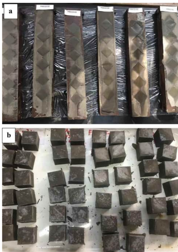
Fig. 4 a Geopolymers molding process and b produced geopolymers cubes
