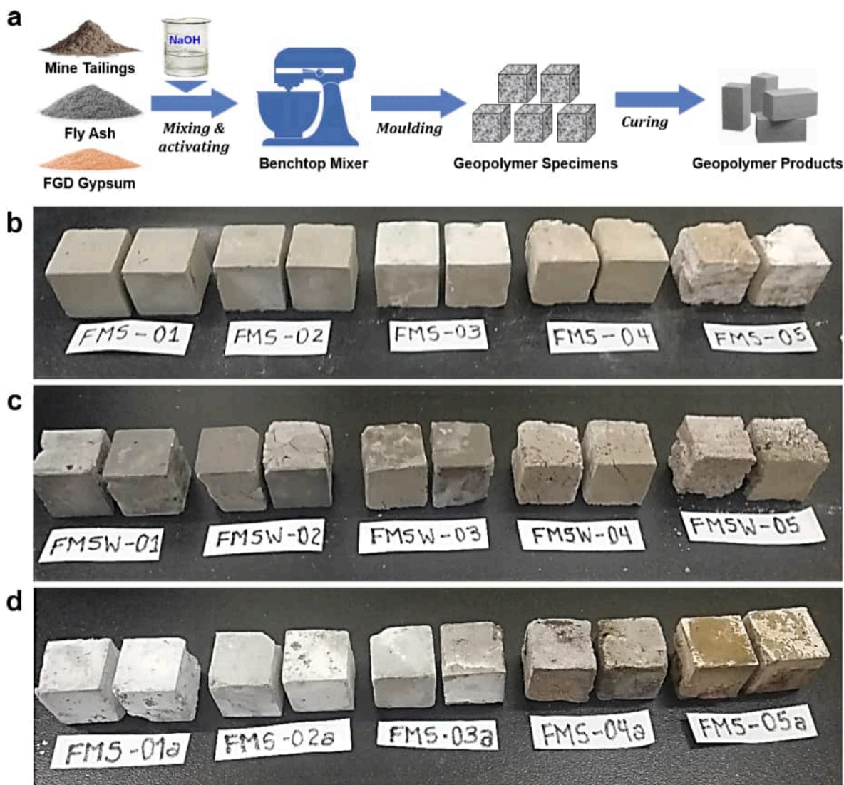
Fig. 2. (a) Schematic illustration of the geopolymer preparation procedure; (b–d) Visual inspections (digital images) of the as-prepared geopolymer cubes, (b) fly ash-mine tailing-sodium hydroxide (FMS) series, (c) fly ash-mine tailing-sodium hydroxide-waterglass (FMSW) series, and (d) fly ash-mine tailing-sodium hydroxide (10 M) (FMS-a) series after curing for 28 days.
