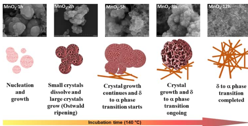
Figure 3. Proposed morphological and phase evolution of the as-prepared MnO 2 with incubation time.
